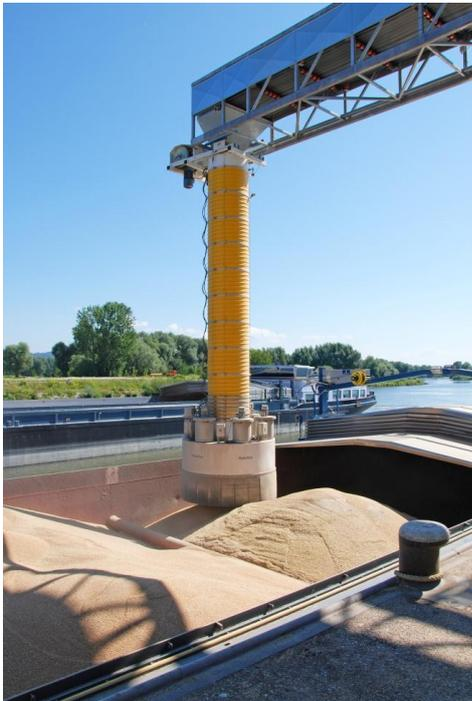
At the end of 2012, BayWa Agrar expanded its grain transfer facility in Regensburg's East Port. The new ship loading facility now has a loading capacity of around 500 tonnes per hour, and the silos can now hold 70,000 tonnes. The capacity for drying
